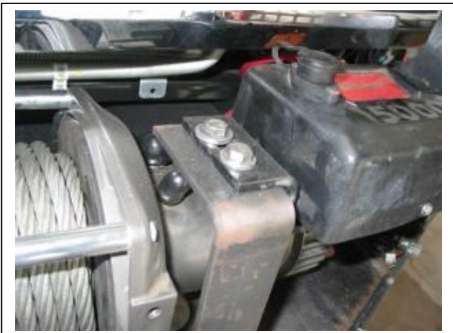
Figure 5: Direction and mounting of winch control box
