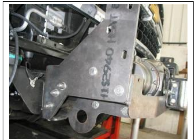
Figure 6: Mounting of winch frame to chassis mount
