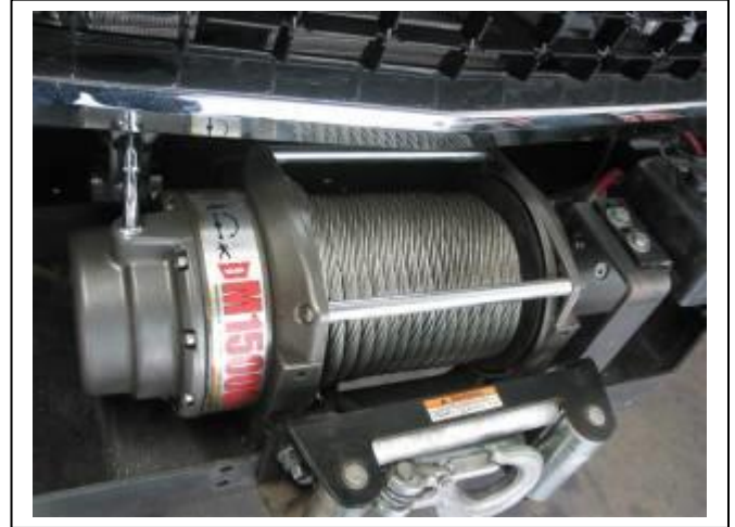
Figure 4: Placement of winch in mount
