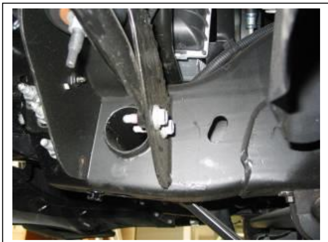
Figure 1: Stay mount to chassis, two 15mm bolts
