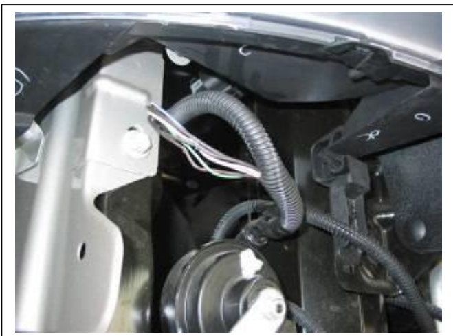
Figure 7: Wiring harness under driver's headlamp
